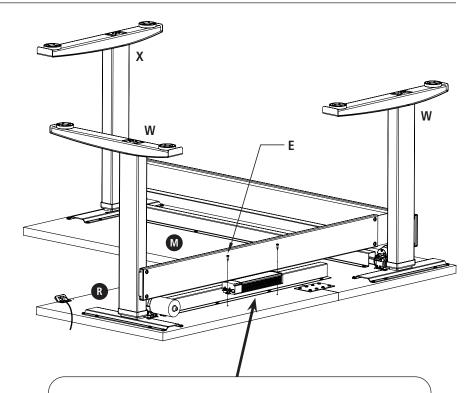
**NOTE:** Table will **NOT** operate unless the control box (T) is screwed tight into the table without any play.
